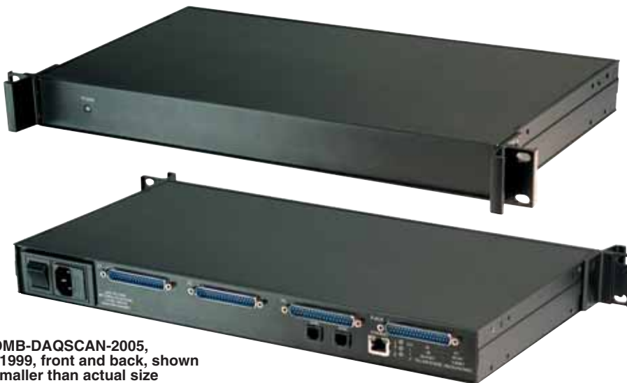
The 80-channel high-speed scanning system consists of an OMB-DAQSCAN-2005 plus five OMB-DBK85 16-channel voltage scanning modules. All channels can be measured at the maximum rate of 5 \mu s/channel.
